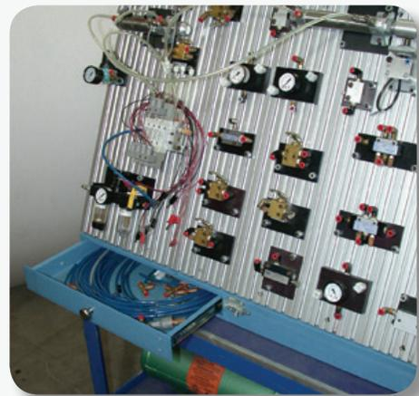
Students will learn to read electrical ladder diagrams, and then create electrical control circuits for the pneumatic systems using solenoid valves as well as switches, relays, timers, counters, LED's and sensors.
